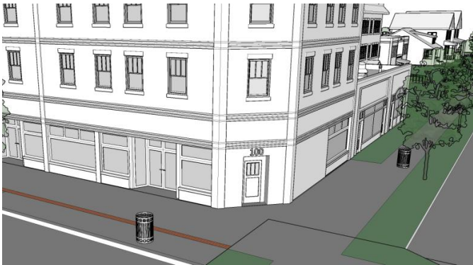
Figure 2.3.D: Example of a chamfered corner
